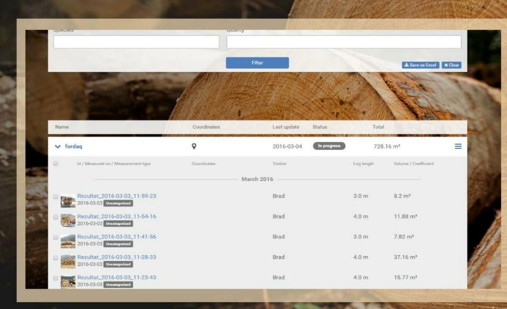
Information can be filtered according to specific storage, date, measurement type or storage status. By clicking on the name of the storage, different measurements stored under this specific storage will open.
